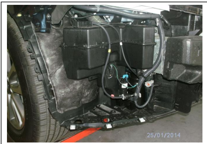
Figure 3: Recommended fog light disconnection point, driver side.
