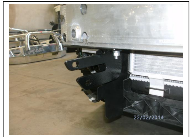
Figure 8: bumper support and mount fitted to vehicle.
