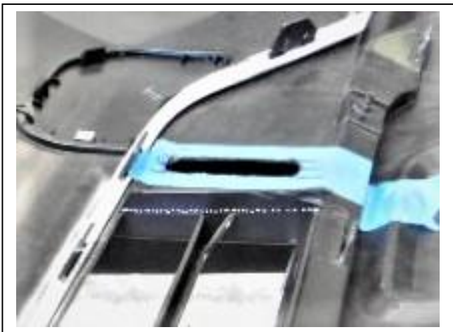
Figure 9: cut areas on drivers side of grille. NOTE: cut area from side of opening.
