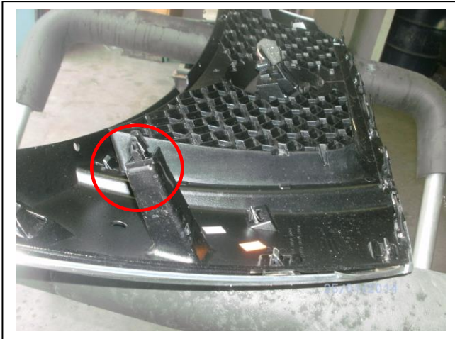
Figure 1: Grille showing placement of top head light mount.
